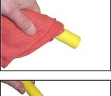
**4b** Chamfer end of pipe using <u>Continental's</u> double ended ID chamfering tool.
