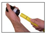
8 Stab pipe completely into fitting so that the mark on the pipe is within 1/8" from the fitting entrance.
